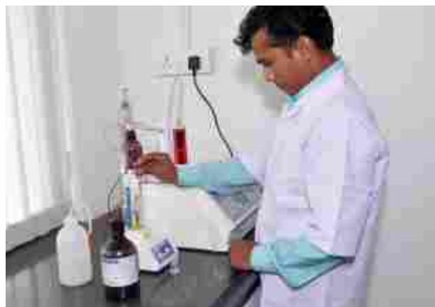
Karl Fischer titration is a classic titration method in analytical chemistry that uses coulometric or volumetric titration to determine trace amounts of water in a sample. It was invented in 1935 by the German chemist Karl Fischer.
